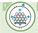
Timber loaded into treatment vessel. Initial vacuum applied and the timber cells are evacuated of air. Vacuum held.
